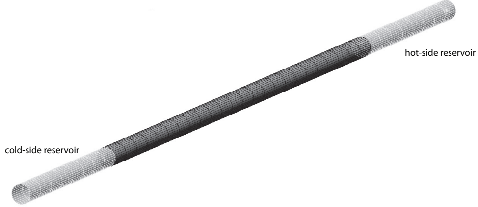
Figure 7.3: Scheme of the numerical domain used for the direct simulation Monte Carlo modeling for the zero-flow case. The micro-tube to which a temperature gradient is applied and the two reservoirs that are kept at constant temperature. The cold-side reservoir is an open boundary kept at constant temperature and pressure while the hot-side reservoir is a closed boundary kept at constant temperature.
